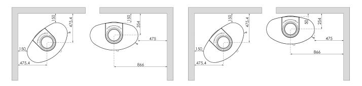
In order to avoid discolouration of painted and treated surfaces, TermaTech recommends the same distance from flammable materials as for non-flammable materials. This distance increases the convection itself around the stove and also eases cleaning. All distances relate solely to the distance of the stove from flammable materials. No account has been taken of national requirements for the use of stove flues or their distance from flammable materials.
