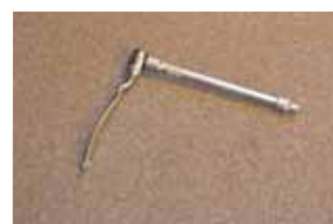
16: Take a number 10 spanner with an extender on a ratchet spanner and stick it down from above through the steel platform.
