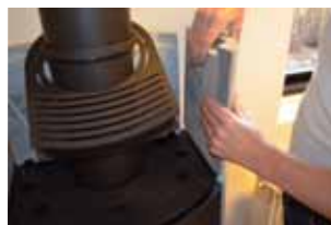
12: Now mount the 2 side stones in the same way as in point 11. BE CAREFUL THAT THE STONES DO NOT FALL DOWN.
